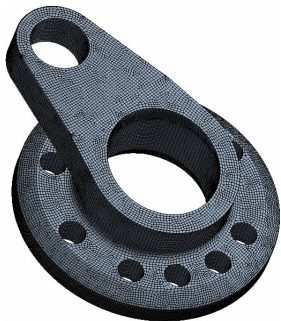
图 10 拐臂有限元网格 Fig.10 Finite element grid of connecting lever
