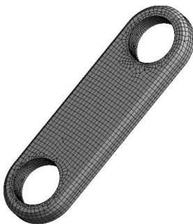
图 9 连杆有限元网格 Fig.9 Finite element grid of connecting rod
